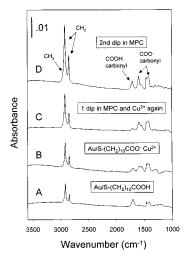
Figure 3. FTIR-ERS spectra showing attachment of Au C6/C5COOH MPCs (  $\sim$ 35/18) to a Au/MUA surface using Cu<sup>2+</sup> linkers; soaking steps indicated in the figure.
