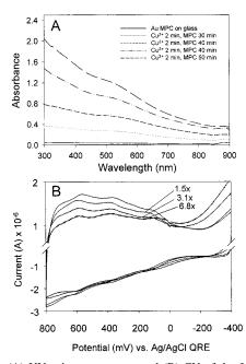
**Figure 2.** (A) UV–vis spectroscopy and (B) CV of the formation of Au C6/C10COOH MPC ( $\sim$ 46/7) multilayers using Cu<sup>2+</sup> linkers, on glass and Au, respectively. In (B), lower to upper curve, 5 min. Cu<sup>2+</sup> exposures followed by 20, 50, 40, 30 min. MPC exposures; current scales of earlier film-forming cycles expanded for comparison. Voltammetry conditions as in Figure 1 except 100 mV/s.
