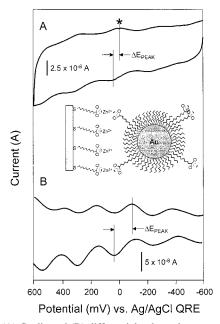
Figure 1. (A) Cyclic and (B) differential pulse voltammetry of Au C6/C10COOH MPCs ( $\sim$ 48/5) attached with one dipping cycle to a Au (0.02 cm<sup>2</sup>)/MUA substrate as illustrated. DC potential scan rate 50 mV/s, 0.1M Bu<sub>4</sub>NPF<sub>6</sub>/CH<sub>2</sub>Cl<sub>2</sub>.
